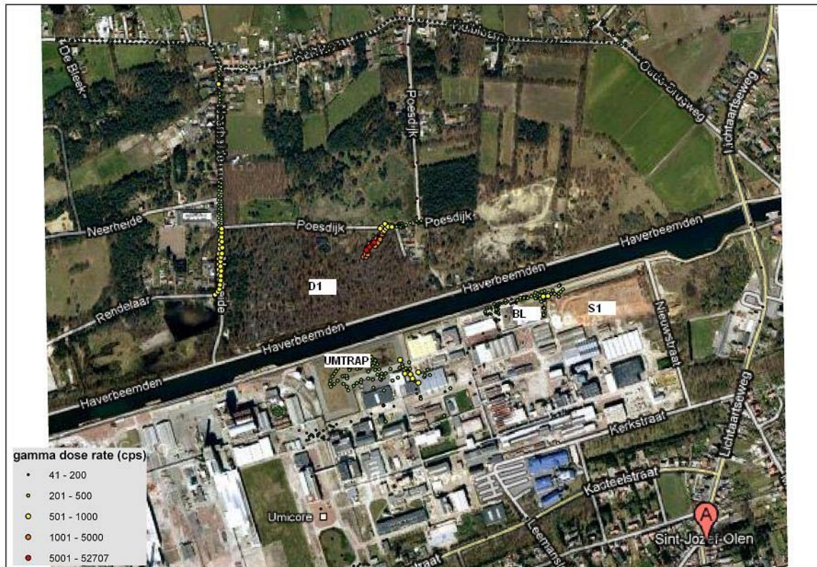
Fig. 5: external radiation (in counts per second) on the surface of the area in Olen.
