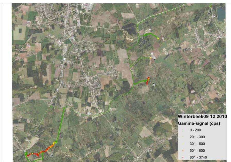
Fig. 1: measurements of gamma radiation (in counts per second) along the banks of the Winterbeek river.
