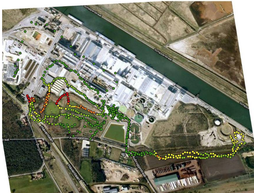
Fig. 4: measurements of gamma radiation (in counts per second) on the surface of the site of TESSENDERLO CHEMIE facility located at Ham
