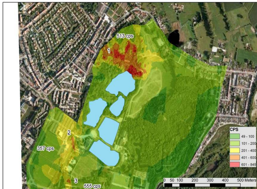
Fig. 6: measurements of gamma radiation (in counts per second) on the surface of the site of the provincial domain "DE SCHORRE" at Boom
