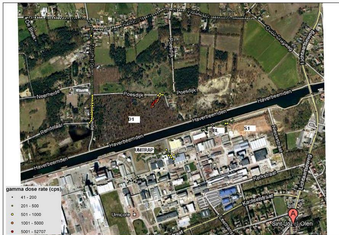
Fig. 8 : external radiation (in counts per second) on the surface of the area in Olen.
