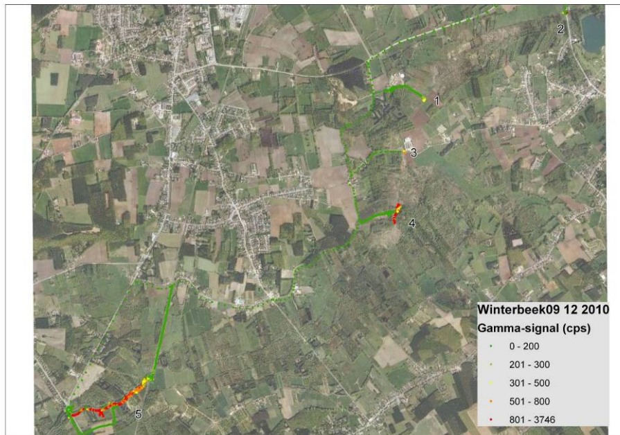
Fig. 1: measurements of gamma radiation (in counts per second) along the banks of the Winterbeek.
