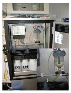
The water is automatically sampled by independent collectors (PPMOS) installed in the containers of the TELERAD river station (photographs opposite).
