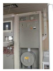
right shows the detector in its casing (cylinder) and the parallelepipedal tube containing the active charcoal cartridges (on the right).
