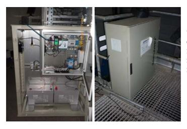
these stations also have a LaBr<sub>3</sub> detector which is coupled to a multichannel detector. Ten radionuclides are defined in the recognition software.
