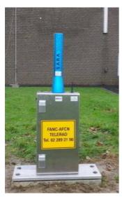
The 64 gamma spectrometry stations (NaI detector) for measuring the ambient gamma radioactivity and the gamma radioactivity of some radionuclides (10 predefined nuclides), are localized on the fences around nuclear sites of SCK•CEN, nuclear power stations of Tihange and Doel as IRE. Photographs show a station in its environment.
