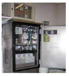
To the left of the gamma spectrometry unit is a large volume water sampler (SwedMeter type) which enables a sample of the water in the pipe to be taken automatically as soon as an alarm level is exceeded. This water is stored in a 25-litre flask for the purpose of subsequent gamma (and beta) spectrometry analyses in the laboratory.
