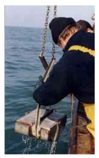
The sediments are brought to the surface using a "Van Veen" scoop (photo on the left), a sort of grapnel with an open jaw lowered to the sea bottom at the end of a steel cable.
