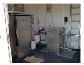
On the far left of the photograph, a programmable automatic sampler (Buhler type PP MOS) enables water to be pumped into flasks for gamma, alpha and beta spectrometry (for the programme for the radiological monitoring of the territory).
