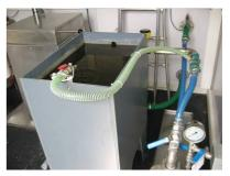
collect suspended particles in the water via a bypass on the water pumping circuit of the TELERAD stations.
